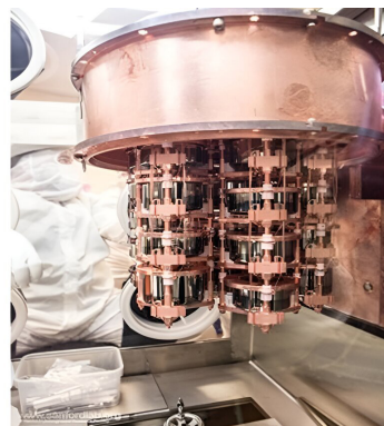
Final assembly of germanium radiation detectors for the Majorana Demonstrator in 2015. These detectors produced a low-background, “quiet” data set that researchers used to search for signs of dark matter and other physics beyond the Standard Model. Credit: Matthew Kapust, Sanford Underground Research Facility.
