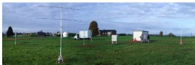
Figure 1 – Picture of the BRAMS radio interferometer in Humain. The five Yagi antennas are visible along the two orthogonal axes.
