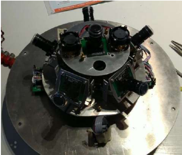
Figure 4 – AllSky6 camera without the dome.
