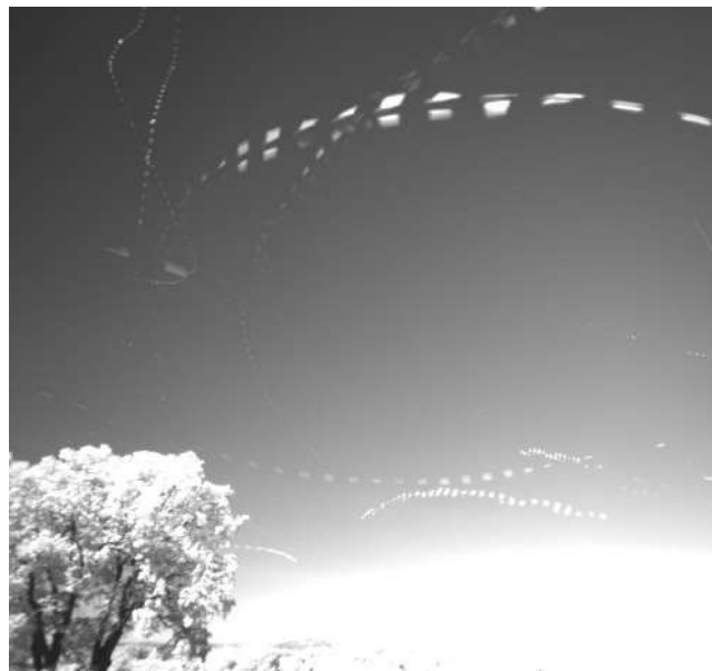
Figure 2 – Typical false detections caused by birds and insects, PFN38 Podgórzyn, DMK33GX174 with IR720 filter
