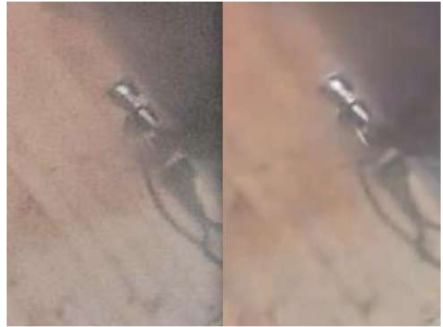
Figure 5 – Two close ups of an image detail in MotionJPEG format (25 Gb/hr), and H.264 (0.4 Gb/ hour).
