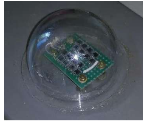
Figure 4 – Matrix of 4x4 BPW34 photodiodes
