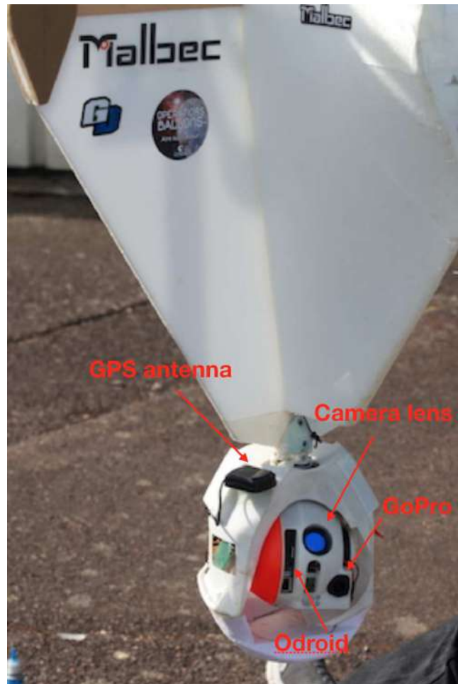
Figure 1 – The 3-axis stabilised MALBEC gondola in 2019.
