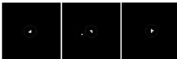
Figure 1 – Test on individual particles to check the algorithm behaviour. The linear correlation between pixels movement and time demonstrates a correct characterization of the physical movement of the particles.
